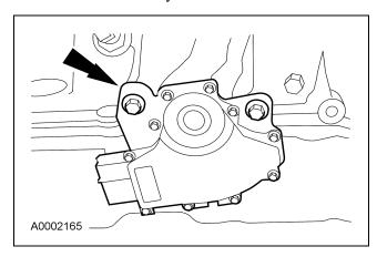
110. CAUTION: Tightening one screw before tightening the other may cause the sensor to bind or become damaged.
